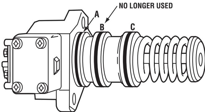
**NOTE:** A change in production has resulted in the removal of the CENTER O-RING on E-Tech unit pumps. It has also been removed from this kit. When assembling O-Rings to pump, install the thicker O-Ring on the bottom groove (position C), the other O-Ring being installed on the top groove (position A). Be sure to lubricate with clean motor oil to ease pump installation.
